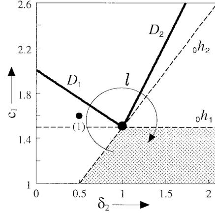
**Fig. 2** Bifurcation diagram of equilibrium points and periodic solutions in Eq. (2) where  $B = 0$ . Dashed and solid lines indicate Hopf bifurcation of the equilibrium point at the origin and D-type of branching of periodic solutions, respectively.
