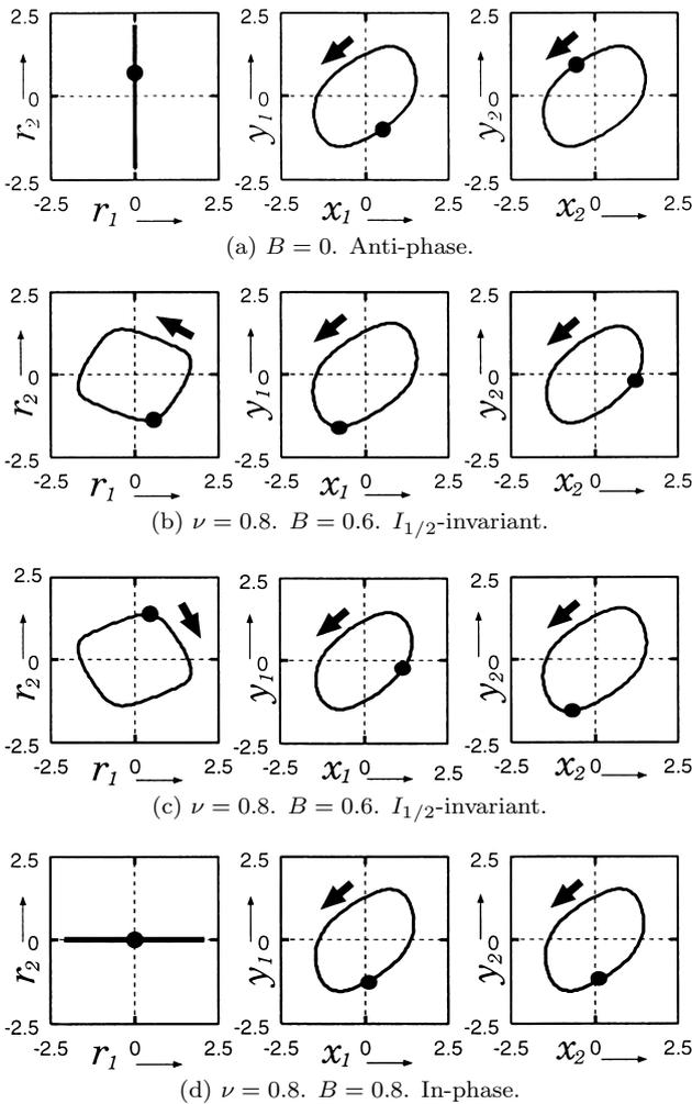
**Fig. 4** Trajectories of the solutions in Eq. (2). Arrows and the points marked by closed circles indicate the time direction of the trajectory and the fixed point of Poincaré map, respectively. (Left)  $r_1$  vs.  $r_2$ . (Middle) Oscillator 1. (Right) Oscillator 2.
