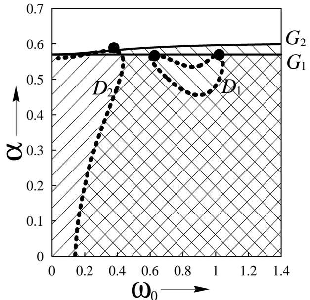
Fig. 2. Bifurcation diagram observed in Eq. (1) with  $\omega = 1.0$ . The subscripts 1 and 2 of  $D$  denote the bifurcation sets of the symmetrical in-phase and the symmetrical partially anti-phase periodic solution, respectively.
