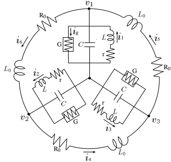
Fig. 1. Circuit diagram. The characteristics of the boxed nonlinear conductance are assumed as  $i_g(v_i) = a_1v_i + a_3v_i^3 + a_5v_i^5$ .
