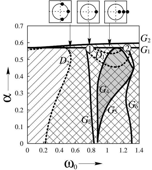
Figure 2: Bifurcation diagram. The subscript 1 and 2 denote the bifurcation sets of the in-phase and the anti-phase solution, respectively.  $G_3$  to  $G_6$  are tangent bifurcation sets of the almost in-phase solution generated by D-type of branching  $D_1$  of the in-phase solution. Small squares above the bifurcation diagram represent the location of characteristic multipliers in a complex plane.
